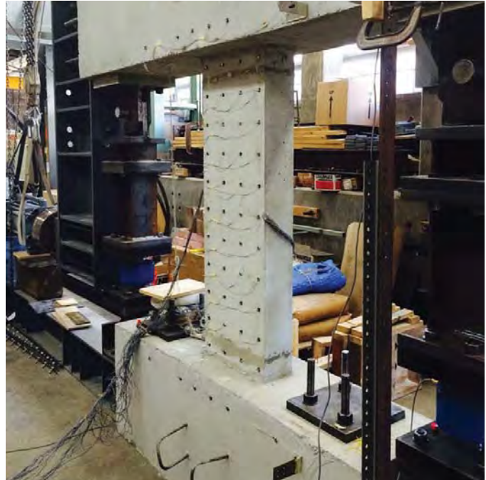
Figure 14. Current SFRC testing. © Gustavo J. Parra-Montesinos & Angel Perez-Irizarry
