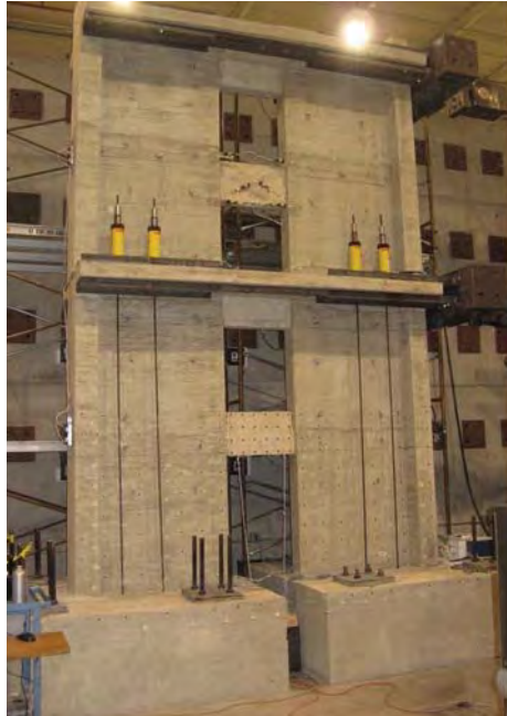
Figure 10. Coupling beam testing at the University of Michigan. © Rémy D. Lequesne.
